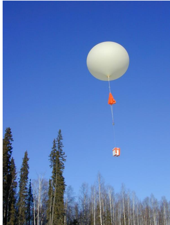
Photo: ECC Ozonesonde being launched in Fairbanks, Alaska. Photo courtesy of NOAA/ESRL Global Monitoring Division.
