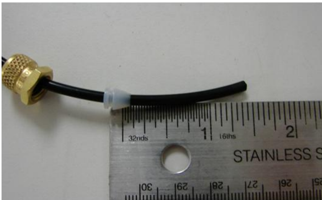
Figure 8: Extra Tubing on Inlet Line
