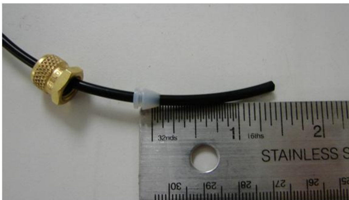
Figure 8: Extra Tubing on Inlet Line
