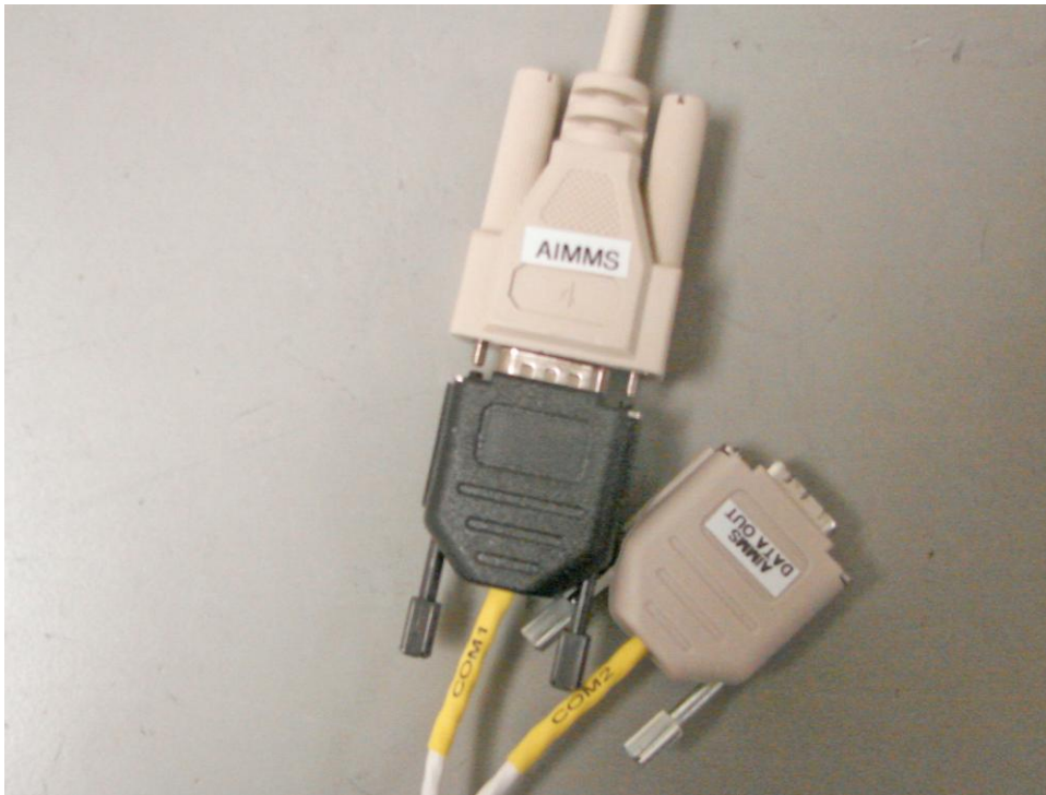
Figure 10: AIMMS20 Data Cable Connection during Configuration
