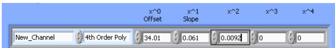
Figure 2: Example Channel Specifications in the Config Editor Window
