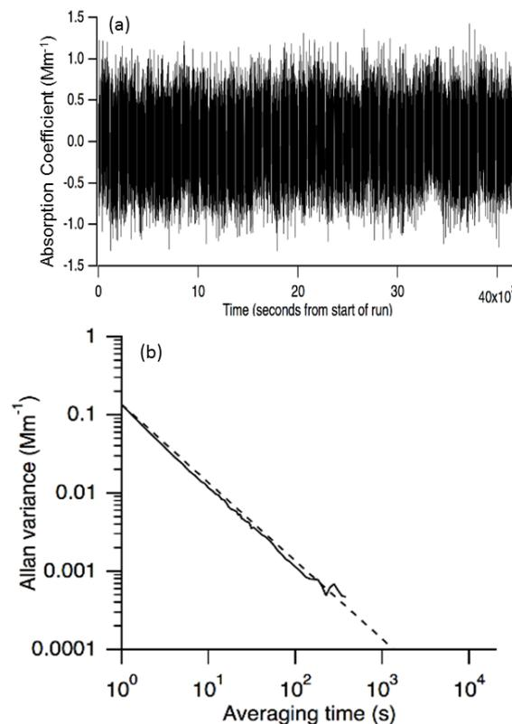
**Figure 3.** Background-corrected absorption coefficients (a) and Allan variance (b) measured by an 870 nm PAX sampling filtered laboratory air overnight in a temperature-controlled environment. The dashed line in (b) gives the variance for white noise.
